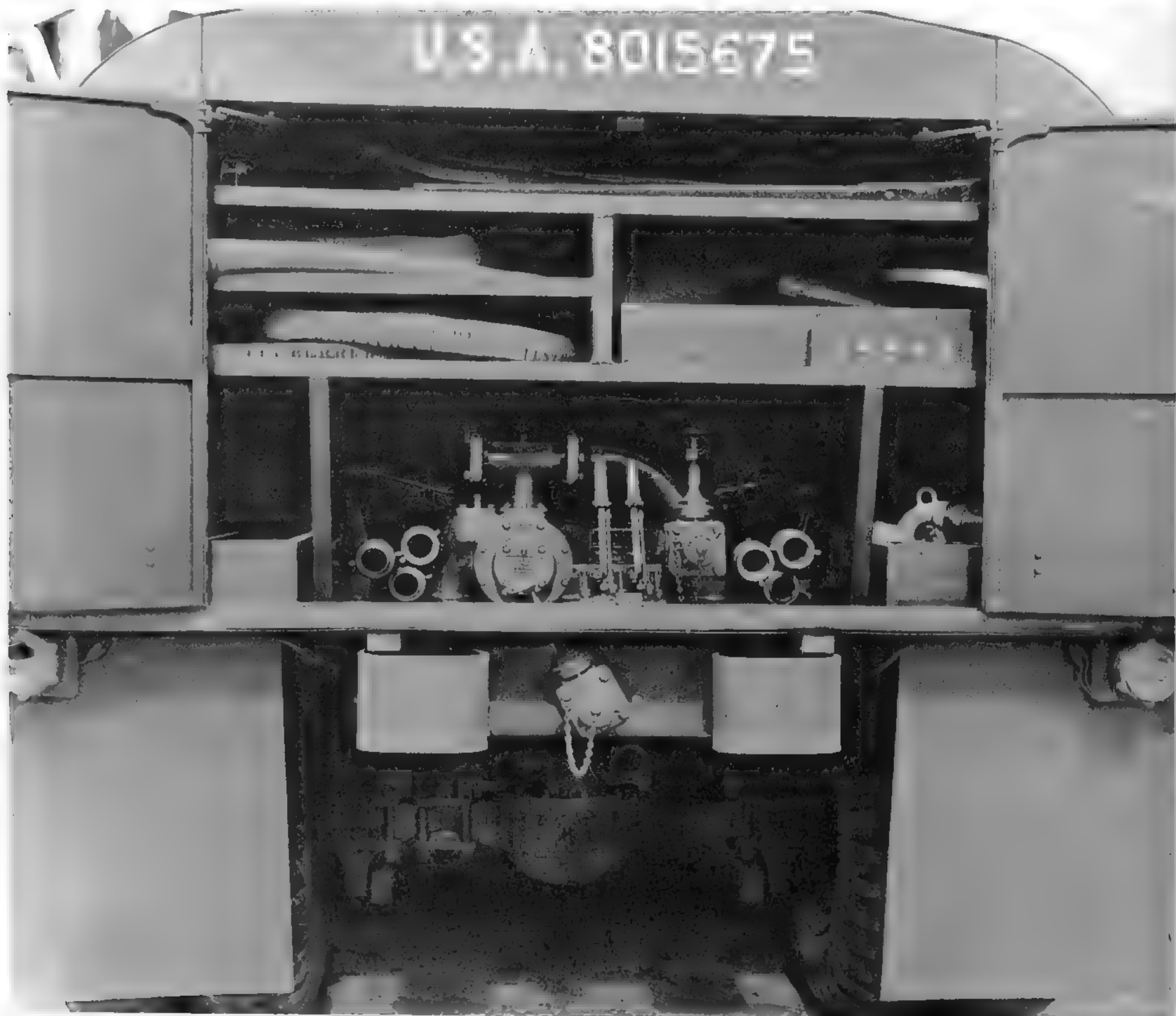
Like the M49, the M50 trucks had the pump assembly in the rear compartment. (National Archives and Records Administration photo)
